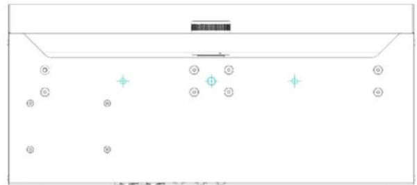
▲The bottom plate of the 4000 series - 1/4" UNC in the middle and M6 screw holes
